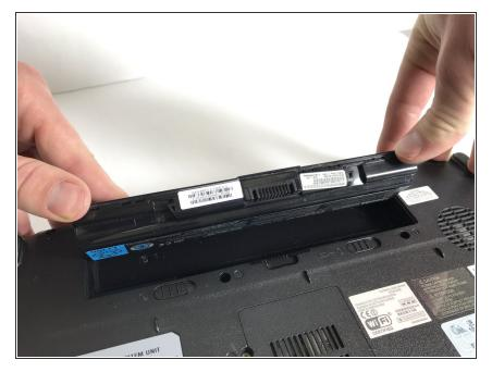
Using a finger or small prying device, pull the battery upwards from the recessed area. Then, simply pull the battery out of the notebook and gently set it aside.
