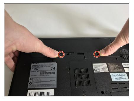
Push the two plastic tabs retaining the battery into the chassis to each respective side. This will push the battery up slightly and release it from the bottom of the notebook.
