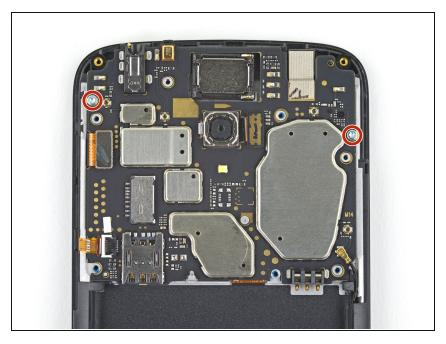
Remove the two 3 mm-long T5 Torx screws securing the motherboard to the phone's frame.
