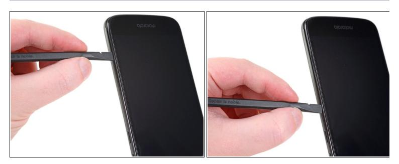
Continue sliding your fingernail or spudger along the seam around the rest of the phone to release the remaining clips.
