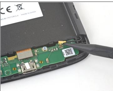
Use the point of a spudger to pry up and disconnect the antenna cable from the daughterboard.
