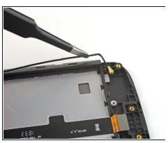
Use your fingers or a pair of tweezers to lift and de-route the antenna cable from its groove on the right edge of the phone.
