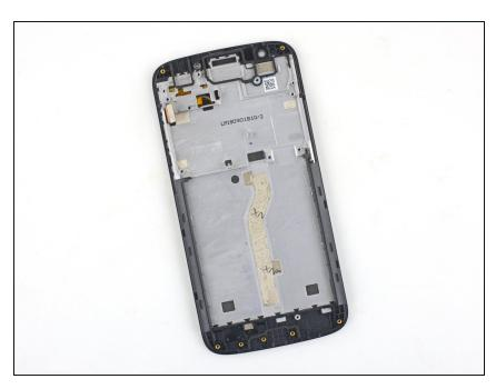
Only the frame and the LCD screen and digitizer assembly remain.
