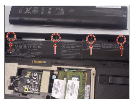
There are four 1.2mm screws under the battery that are needed to be removed with a Phillips screwdriver.
