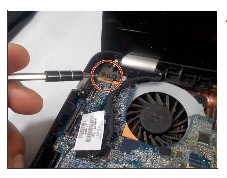
Unscrew the two 3mm screws beside the fan with a Phillips screwdriver.
