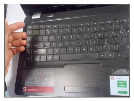
Turn the laptop back, and open the laptop cover. Use a spudger or your hand to carefully remove the keyboard.
