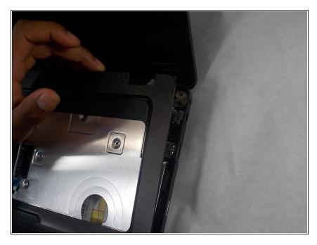
Once the keyboard is out, use the Metal Spudger or your hand in the corner of the laptop to lift the outside frame.
