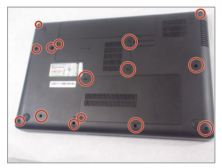
Turn the laptop upside down, and unscrew all the 3.0mm screws on the back cover with a Phillips screwdriver.
