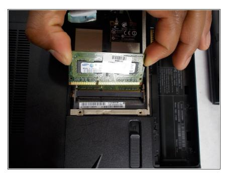
Insert your new RAM replacement into the slot where the old one was removed. Push until you hear a small click.
