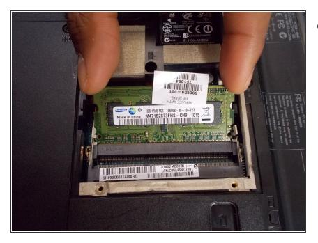
To remove the RAM, start by lifting up the first card. Grab each side of the card with two fingers as shown in the picture and pull gently until it is removed from its slot.
