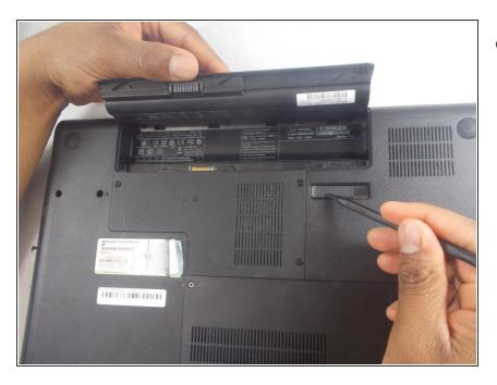
Remove the battery by pushing the lock to the left and lifting the battery from its socket.
