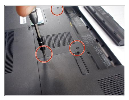
Once the battery is out, locate a panel that is underneath the battery compartment and unscrew the three 3mm screws with a Philips screwdriver.
