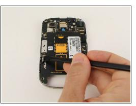
Use the black nylon spudger to pop the press fit connector up from the lower left corner of the motherboard.
