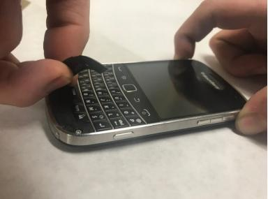
• Lift the bezel at the bottom of the phone up and peel it away from the phone.
