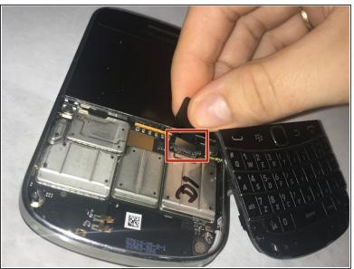
The keyboard is attached via a ribbon cable. Pull the cable up to remove the keyboard.
