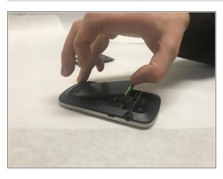
Lift the edge of battery with the green stripe upward to remove battery.
