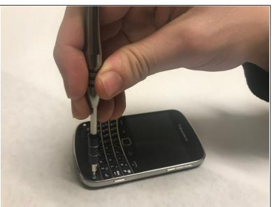
Remove the two exposed screws using the T5 Torx screwdriver.
