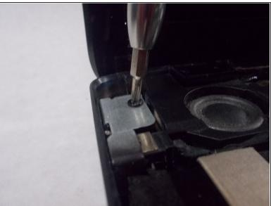
Remove the one 7 mm screw located at the top left corner of the laptop near the charging port using the Phillips #0 screwdriver.
