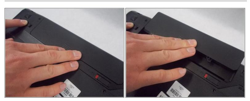
Push the battery forward lightly to remove it while holding the left switch.
