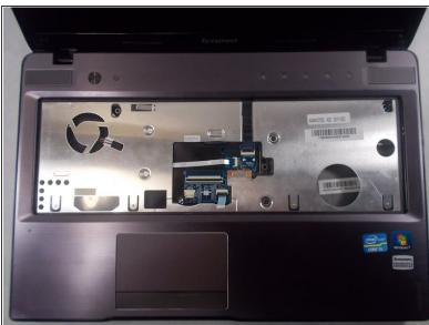
Pull the keyboard out from the terminal block.
