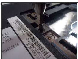
Remove the three 12mm screws found near these symbols with a Phillips #0 screwdriver.
