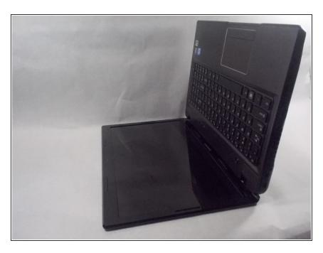
Orient the laptop at a 90 degree angle with the keyboard being vertical and the screen horizontal to the surface you are working on.
