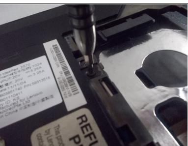
• Remove the 3 mm Phillips #0 screw located on the left hand side that holds the disc drive in place.
