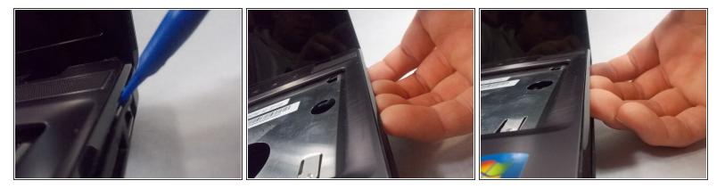
Wedge the opening tool between the ethernet jack and the speaker to pry of the front plate of the laptop.
