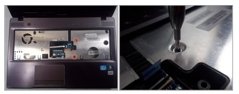
Remove the two 7mm screws found on the right side of the silver plating on the laptop using the Phillips #0 screwdriver.
