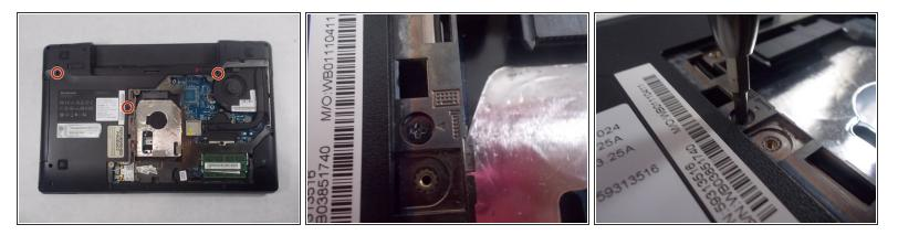
• Remove the three 12mm screws found near these symbols with a Phillips #0 screwdriver.
