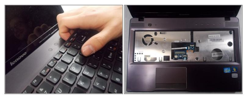
• Pull the keyboard out from the terminal block.
