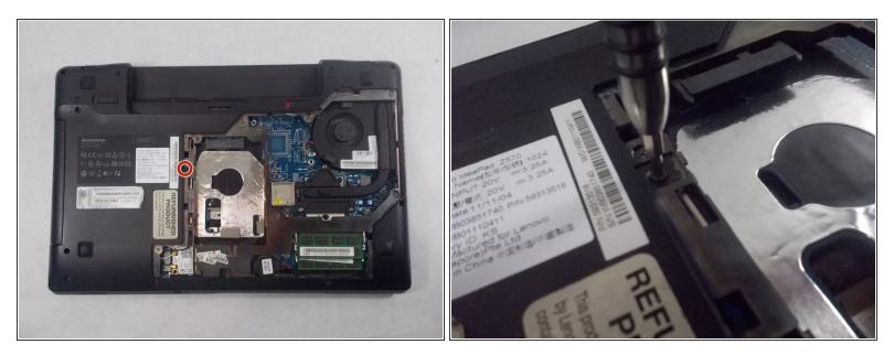
• Remove the 3 mm Phillips #0 screw located on the left hand side that holds the disc drive in place.
