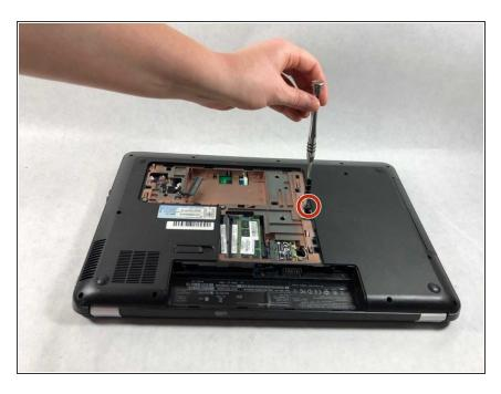
Use the screwdriver to remove the 4mm Phillips #0 screw holding the optical drive in.
