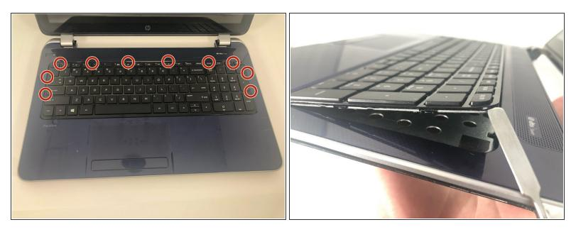
Use the metal spudger to release the keyboard from the front panel.
