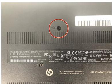
Unscrew the 6 mm Phillips #1 screw securing the keyboard.
