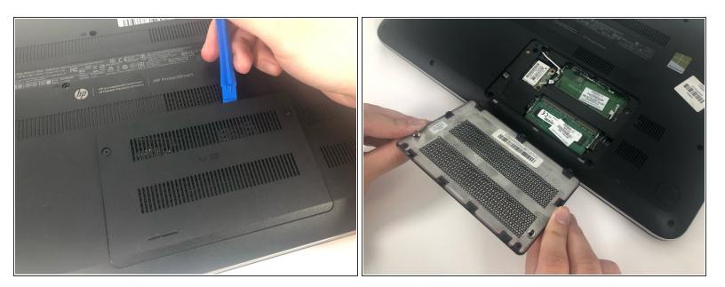
• Use the iFixit opening tool to remove the back panel.
