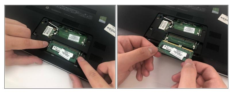
• Release the clips securing the RAM by slightly bending them until the RAM is free.
