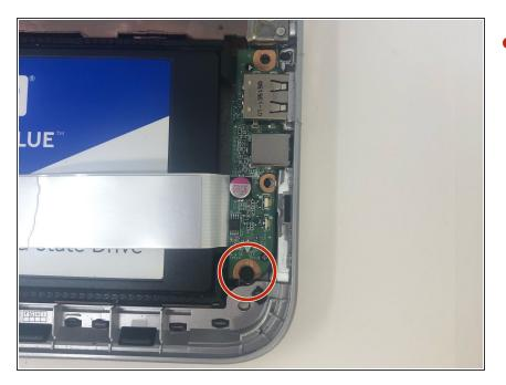
Remove the 2.5 mm Phillips #1 screw and remove the daughterboard
