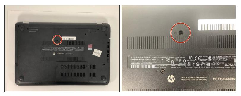
Unscrew the 6 mm Phillips #1 screw securing the keyboard.
