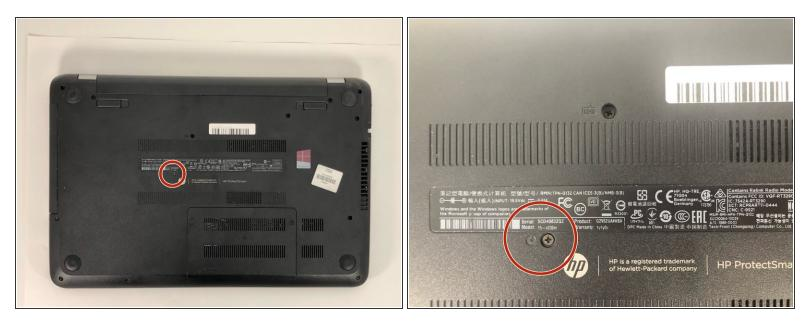
• Remove the 6 mm Phillips #1 screw securing the optical drive.
