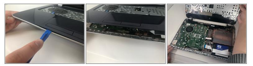
• Carefully use the iFixit opening tool to release the front panel.
