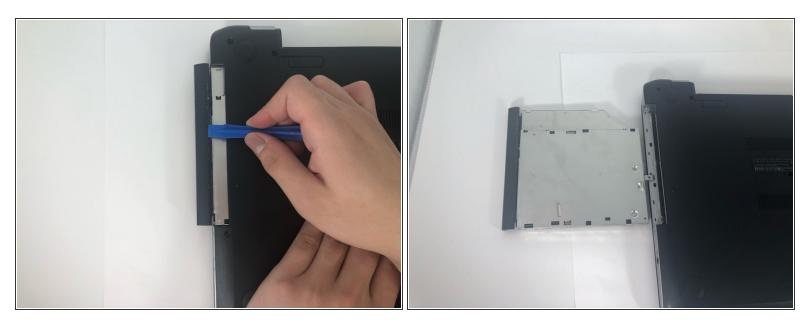
• Use the iFixit opening tool to slide the optical drive away from the laptop housing.
