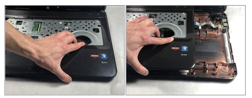
Remove the upper case assembly by lifting it away from the rest of the laptop.
