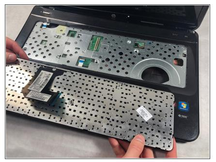
Remove the keyboard from the device.
