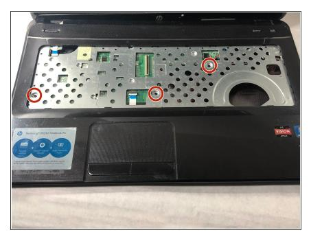
Locate the three Phillips M2.5 x 6.5 on the upper case assembly.
