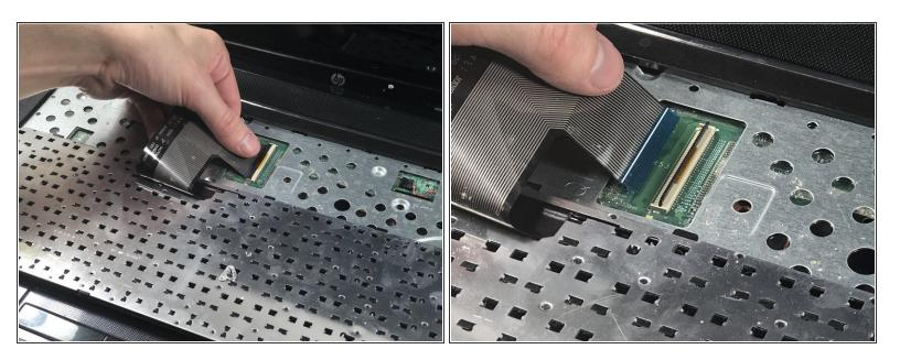
Pull the keyboard ribbon cable out from the connector.
