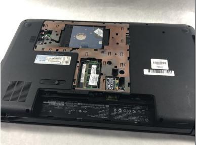
Lift the service door up and away from the device.
