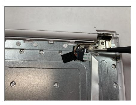
Remove adhesive that secures the ribbon cable using tweezers.
