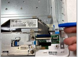
Using a plastic spudger, flip open the switch for the connection port, allowing the ribbon cable to be removed.
