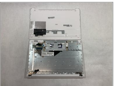
Completely remove the back casing.
