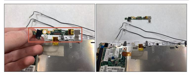
• Using a plastic spudger remove the camera circuit board from the device.
