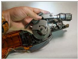
Remove the gear assembly by pulling it straight up.
