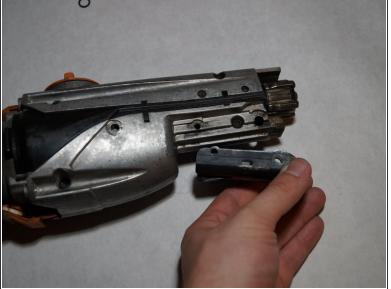
Remove the one 16mm T20 screw that holds the grip support onto the saw.
