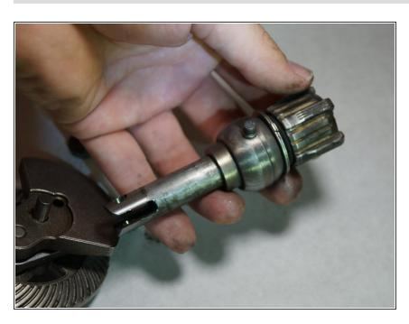
Slide the blade clamp assembly off the gear assembly.
