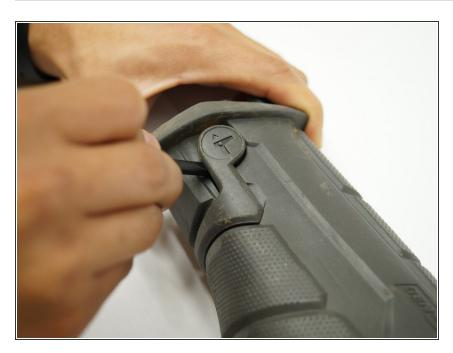
Remove the plastic tab holding the handle cover in place by prying upward with the spudger until the tab pops off.
