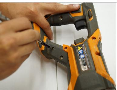
Use a T20 Torx screwdriver to remove the nine M4 X 16mm screws from the plastic housing.
