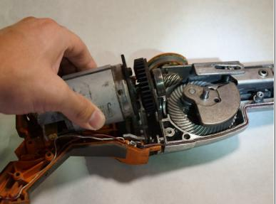
Carefully remove the motor making sure not to harm any of the wires that are attached. Place motor gently out of the way.
