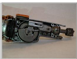
Remove the five T20 Torx screws from the gear assembly cover and pull the cover off.
