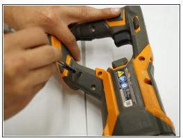
Use a T20 Torx screwdriver to remove the nine M4 X 16mm screws from the plastic housing.
