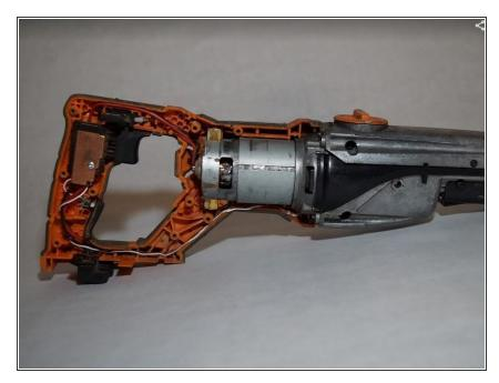
Remove one half of the plastic housing using a spudger so that the internal system is exposed.
