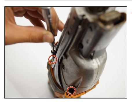
Use a JIS #1 screwdriver to remove the two M4 x 25mm screws on both sides of the metal housing.
