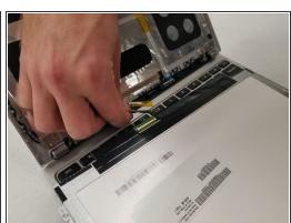
Lift the lever to release the cable and pull the cable out.
