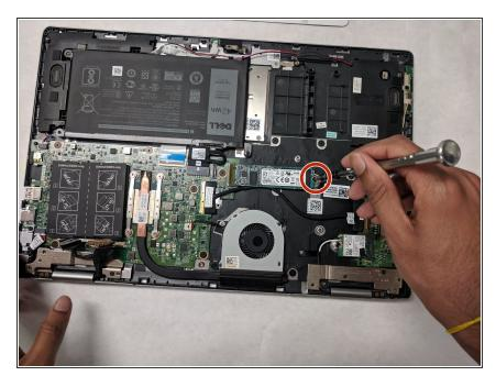
Unscrew the 3.7mm screw that attaches the solid state drive with the Phillips #0 screwdriver.
