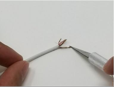
Burn off the insulating wax from the signal carrying wires with a lighter and/or use a knife to rub it off.
