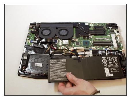
Remove battery from device.
