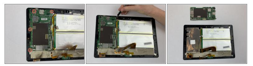
Remove the four black 3.32mm screws on the corners of the motherboard using the Phillips #000 screwdriver. The motherboard should come out easily.
