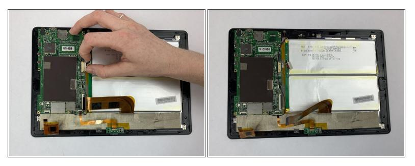
• Disconnect the battery's bundled cable connector from the motherboard with fingers.
