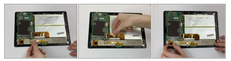
• Gently remove the battery's three ZIF connectors from the motherboard. Use your fingers.
