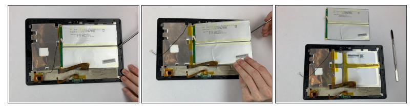
Pry the battery away from the display screen gently using a nylon spudger or the plastic opening tools.
