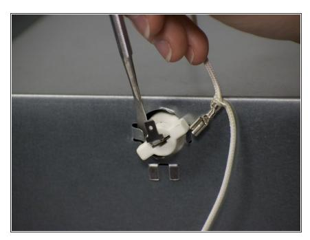
Use a metal spudger to unfold the tabs of metal that hold heating element in place.
