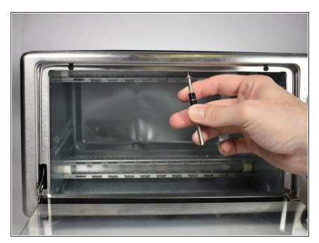
Locate retaining screw on the uppermiddle portion of the door frame.
