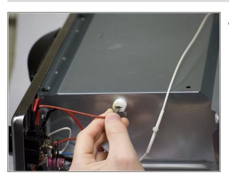
Remove the red wire from the heating element.
