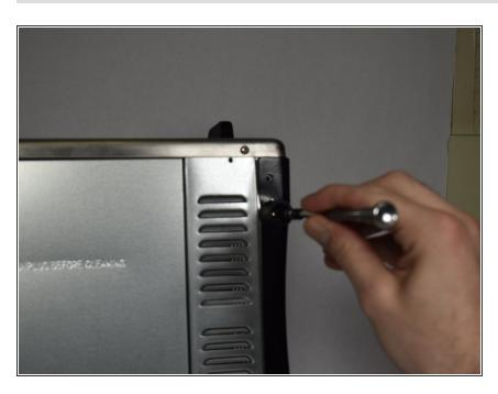
Remove four 13.7mm Phillips #2 screws from black plastic feet to separate the cover from the device.
