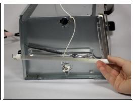
Gently push the heating element from the side with the red wire to remove it from the toaster.
