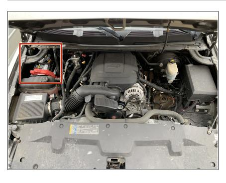
The battery is located in the back left corner of the engine bay, partially covered by an engine bay brace.
