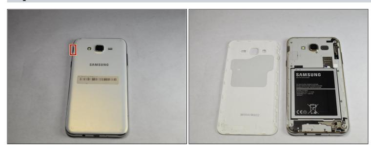
Remove the back of the device by pulling on the tab in the top left.
