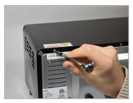
Remove five 11.6 mm Phillips #2 screws from the rear of the device.
