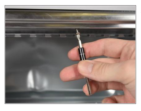
Remove one 21.9 mm Phillips #2 retaining screw from upper-middle portion of door frame.
