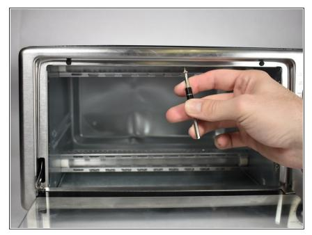
Locate retaining screw on the uppermiddle portion of the door frame.
