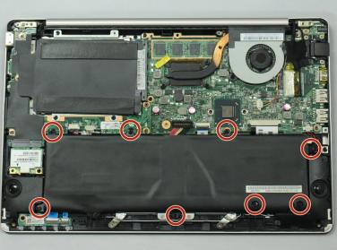
• Remove the eight 5mm screws using a Phillips #1 screwdriver.
