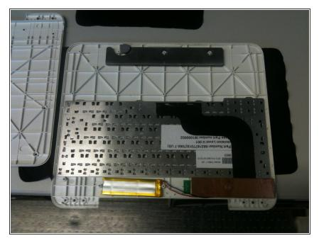
Once the screws are removed, lift off the bottom panel to access the keyboard and battery.
