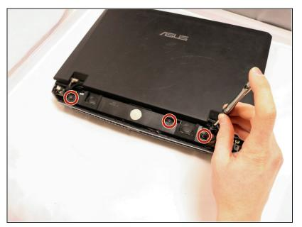
Using the PH 00 screwdriver, remove the three 10.6 mm screws holding the sound bar down.
