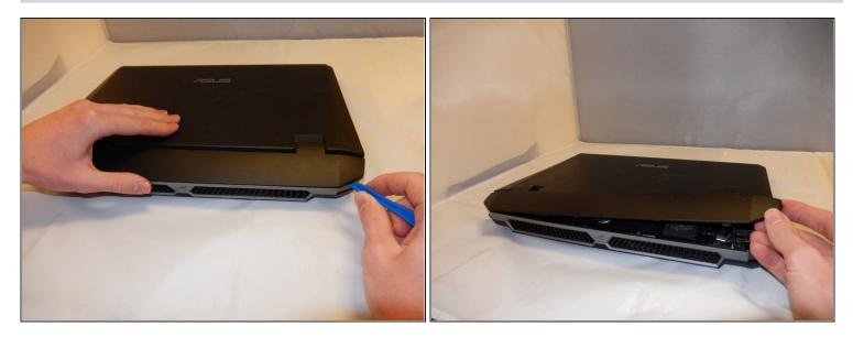
• Using the iFixit opening tool, gently pry open the plate covering the spine of the device.
