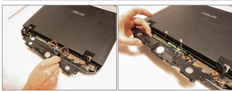
• Using the bent black <u>tweezers</u>, remove both wires connecting the sound bar to the motherboard.
