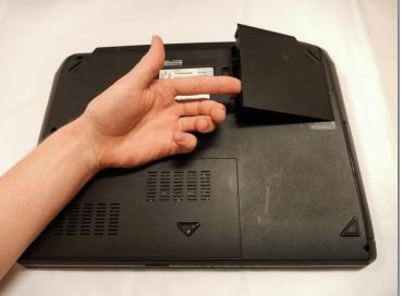
Side the switch and lift the battery from the back of the device.
