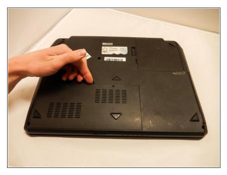
Lift and remove the back plate.
