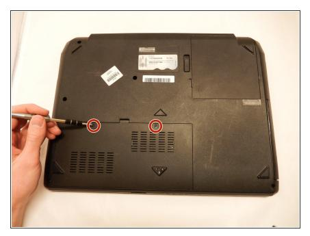
Using the PH0 screwdriver remove the 2 3.6 mm screws.
