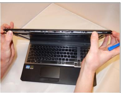
Using your iFixit opening tool, separate the frame by gently prying the two seams apart without completely removing the plastic frame piece.
