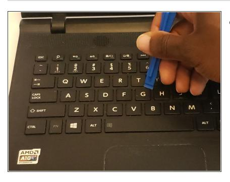
Wedge your ifixit opening tool underneath the non-functioning key.
