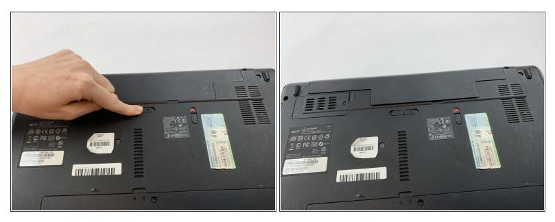
• Pull the other switch completely while the red unlock symbol is still present. The battery pack should pop up a bit.
