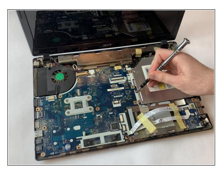
Unscrew the 5.6 mm screws keeping the motherboard in place using a Phillips #0 screwdriver.
