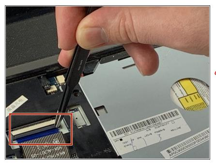
Using tweezers, slide the the tab down. This will release the connector that you can gently pull out of the socket.
