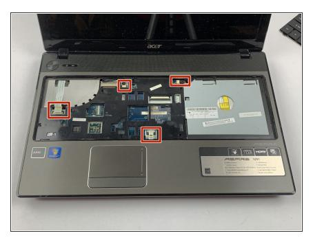
• Locate the 4 connectors that must also be disconnected.
