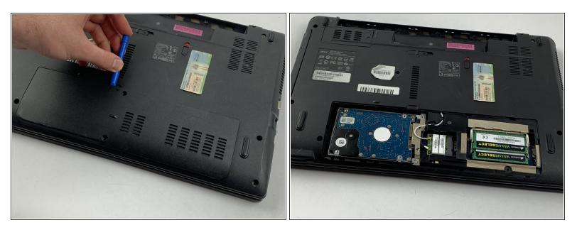
• Using a plastic opening tool, lift up the panel and remove it completely.
