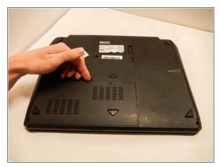
• Lift up and remove the back plate that is located in the back, bottom left portion of the laptop.
