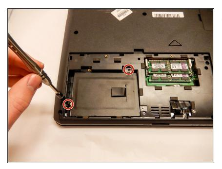
Using the Phillips size 0 remove both 4.6 mm screws from the metal tabs.
