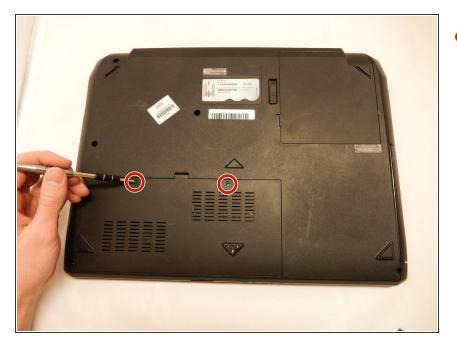
Using the Phillips size 0 head screwdriver, remove the 2 3.6 mm screws on the back plate located on the bottom left portion of the back of the laptop.
