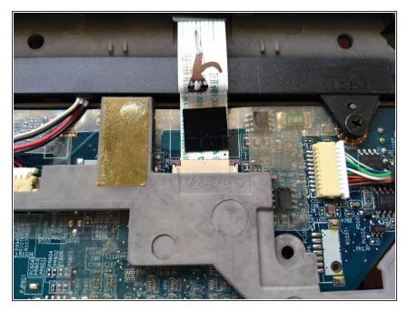
• Before tearing the plastic surrounding the keyboard, remove the ribbon cable holding it in place.
