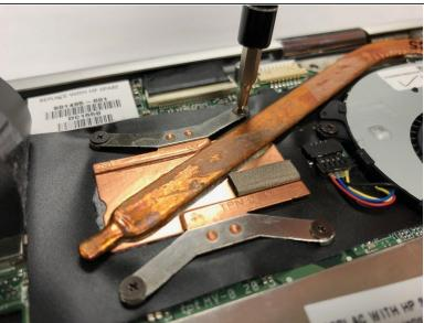
Remove the four 3 mm screws using a Phillips #0 screwdriver.
