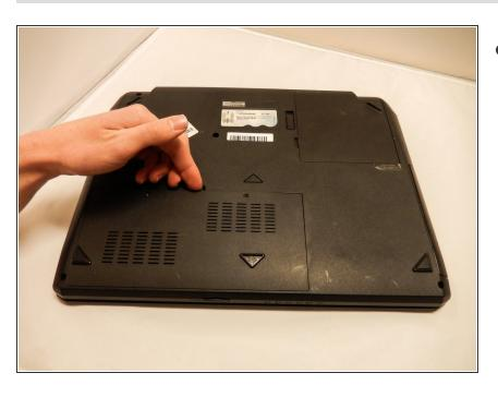
Lift up and remove the back plate from the device.
