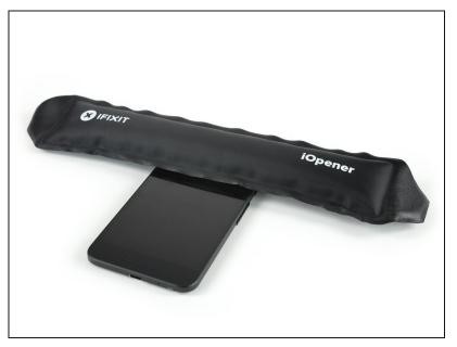
Use an iOpener to loosen the adhesive beneath the rear facing camera. Place the iOpener across the top part of the phone for about 30 seconds.
