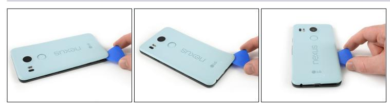
• Continue to slide the opening pick around all sides of the phone to release all clips that secure the rear panel.
