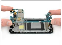
• Grip the lower part of the motherboard with your fingers and carefully lift it upwards.
