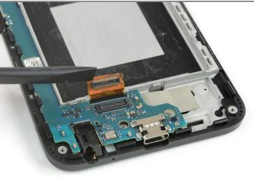
Use the flat end of a spudger to pry up the display flex connector.
