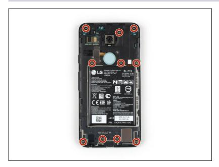
Remove the ten 3.6 mm Phillips screws that secure the midframe.
