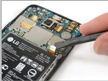
• Use the edge of a spudger to pry up and disconnect the battery flex cable located at the bottom right of the motherboard.
