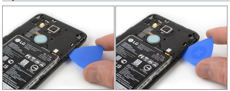
• Insert an opening pick into the SIM card tray slot and twist the opening pick sideways to release the plastic clips.
