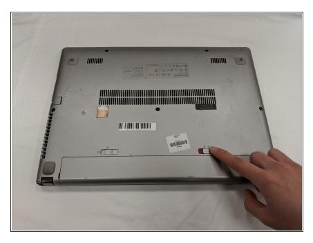
Use your finger to push the battery release switch labeled "1." The red indicates that the switch is unlocked.
