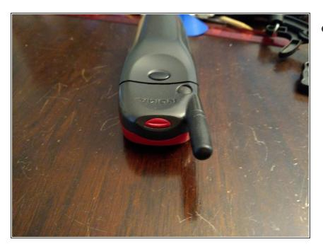
Find the tab at the top of the phone and press down with your fingernail or the flat end of a spudger
