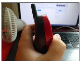
• Make sure the two tabs at the bottom of the cover go into the phone first at an angle, the push the top of the cover in until it clicks and then you are done!
