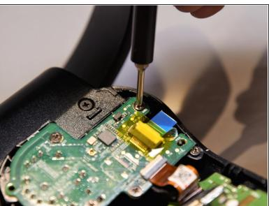
Using a Phillips #00 screwdriver, remove the four 4mm screws located on the joystick circuit board underneath the top half of the controller.
