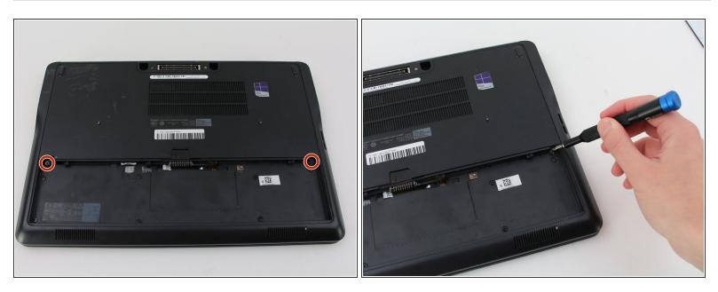
Remove two M2 x 3mm Phillips #0 screws from the base cover.
