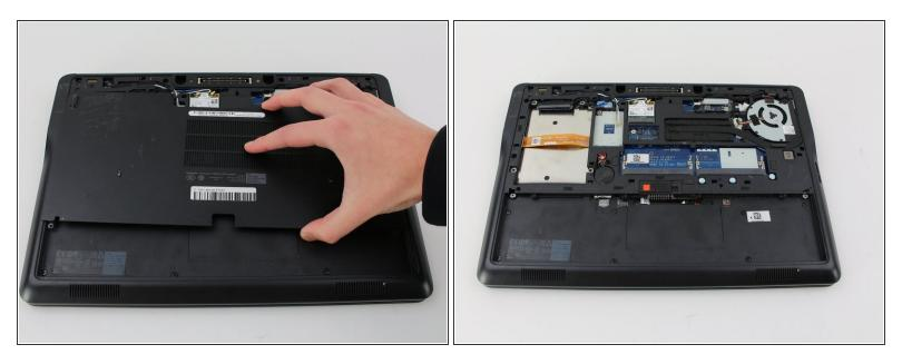
• Slide the base cover down slightly and remove it.
