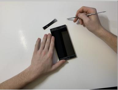
• Pry the top plastic grill off with the metal spudger and reveal the screws.
