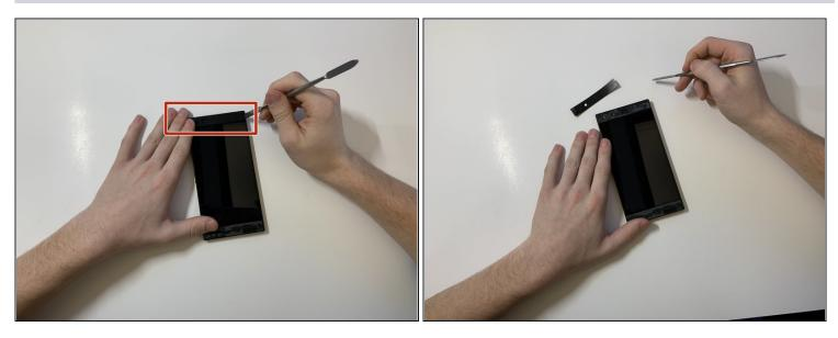
• Pry the top plastic grill off with the metal spudger and reveal the screws.
