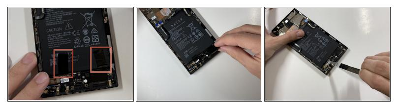
• Peel off and pull out the elastic tabs at the bottom of the battery.
