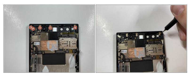
Remove the five 1 mm screws holding down the gold antenna line brackets to the motherboard using the Phillips #000 screwdriver.
