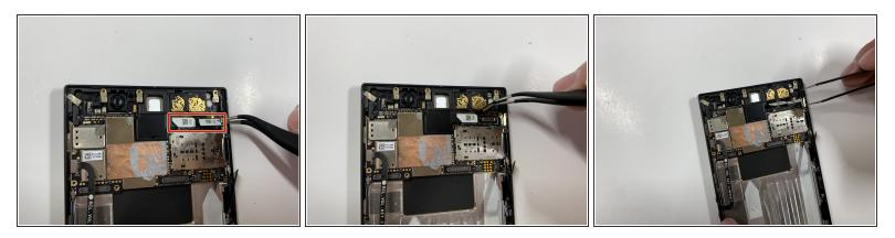
• Grab the connectors with the tweezers and gently lift the connectors loose.
