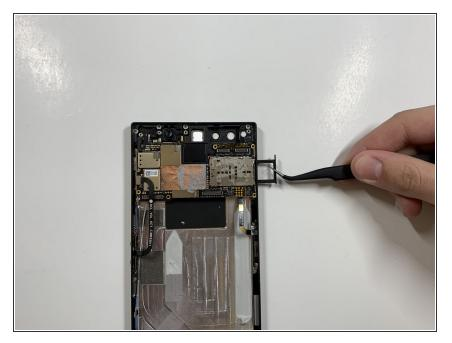
Using the tweezers remove the SIM card tray from the body of the phone.
