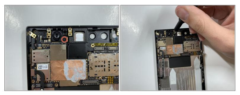
• Remove the 2.5 mm screw next to the front-facing camera with the Phillips #000 screwdriver.
