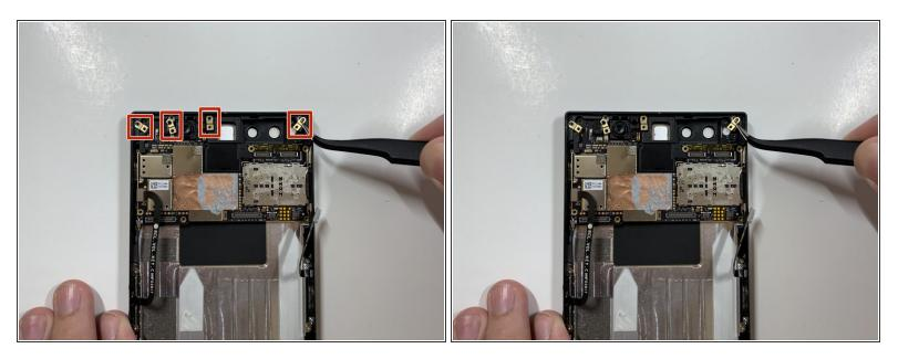
Remove the four gold antenna line brackets with the tweezers.
