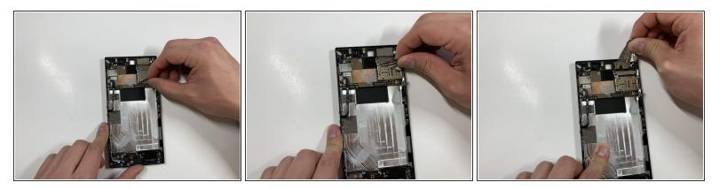
• Remove the protective peel covering the rear cameras using your hands.
