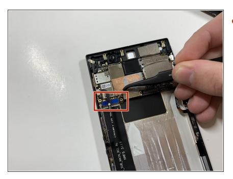
Grab and remove the blue connector with the tweezers.
