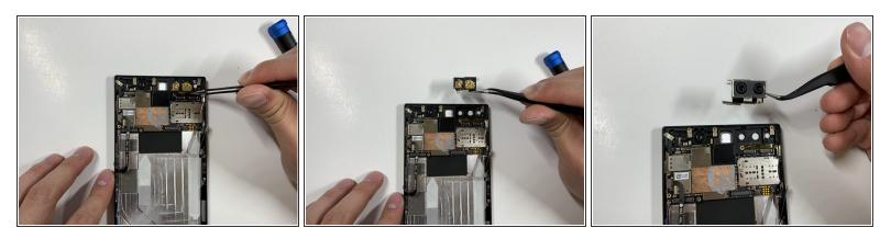
• Grab the loose connectors with a tweezer and gently remove the rear camera unit from the phone.
