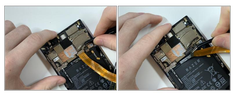
• Grab hold of the the screen ribbon with the tweezers and remove it from the rest of the phone to free the assembly display.
