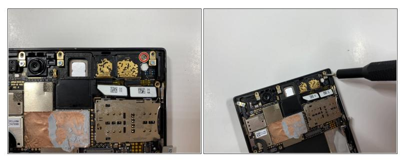
Remove the one 2.5 mm screw with the Phillips #000 screwdriver.
