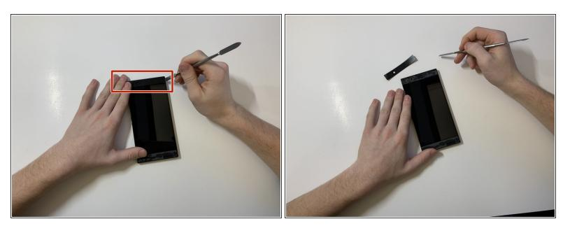
Pry the top plastic grill off with the metal spudger and reveal the screws.
