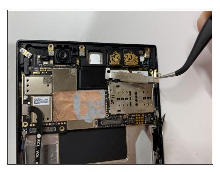
• Grab and remove the metal tab with the tweezers.
