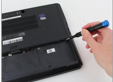
• Remove two M2 x 3mm Phillips #0 screws from the base cover.
