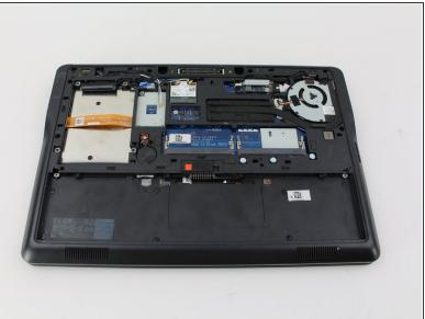
Slide the base cover down slightly and remove it.
