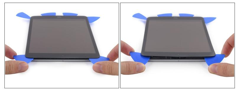
Be very careful with this step. Take your time and ensure the adhesive is hot and soft, and that you've been through all of the adhesive with an opening pick. Don't be afraid to stop and reheat.
