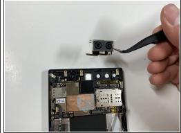
Grab the loose connectors with a tweezer and gently remove the rear camera unit from the phone.
