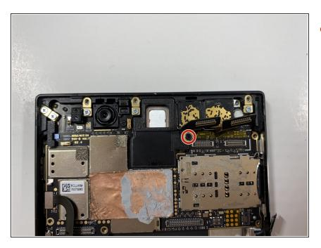
Remove the one 2.5 mm screw underneath the connectors with the Phillips #000 screwdriver.
