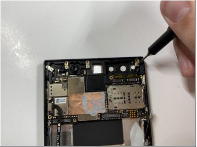
Remove the five 1 mm screws holding down the gold antenna line brackets to the motherboard using the Phillips #000 screwdriver.
