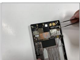
Grab the connectors with the tweezers and gently lift the connectors loose.
