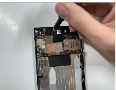
Remove the 2.5 mm screw next to the front-facing camera with the Phillips #000 screwdriver.
