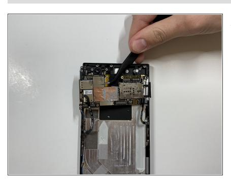
Carefully lift up the motherboard away from the device.
