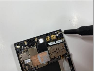
Remove the one 2.5 mm screw with the Phillips #000 screwdriver.
