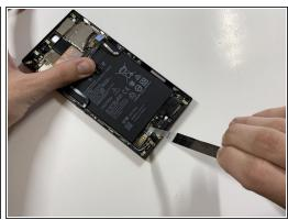
Peel off and pull out the elastic tabs at the bottom of the battery.
