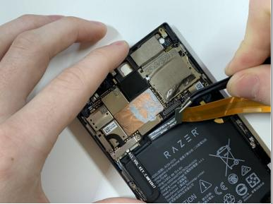
Grab hold of the the screen ribbon with the tweezers and remove it from the rest of the phone to free the assembly display.
