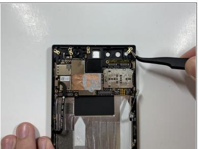
Remove the four gold antenna line brackets with the tweezers.
