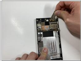
• Remove the protective peel covering the rear cameras using your hands.
