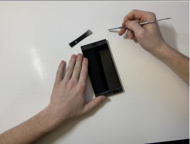
Pry the top plastic grill off with the metal spudger and reveal the screws.
