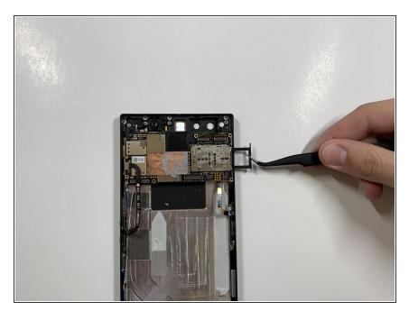
Using the tweezers remove the SIM card tray from the body of the phone.
