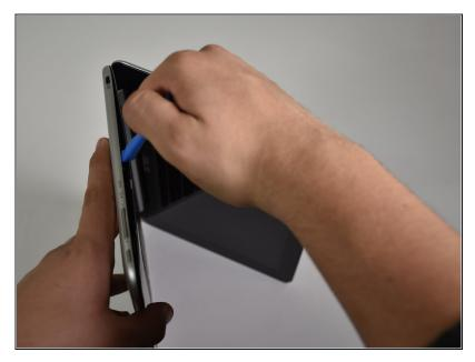
Use the iFixit opening tool to pry the backing of the device off.
