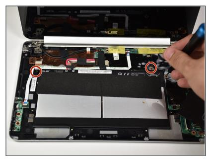
Use the J00 screwdriver to remove the three 1.7 mm battery screws.
