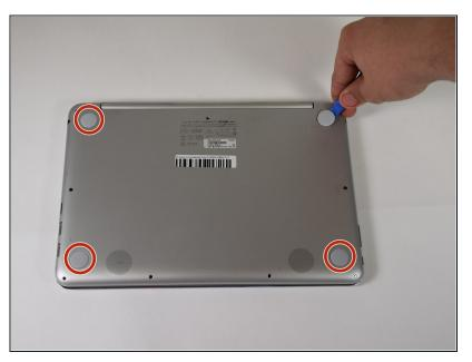
Use the iFixit opening tool to remove the 4 pads to reveal six 3.1 mm screws underneath.
