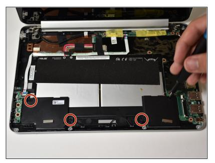
• Use the JIS1 screwdriver to remove the four 2.1 mm screws around the audio cards.
