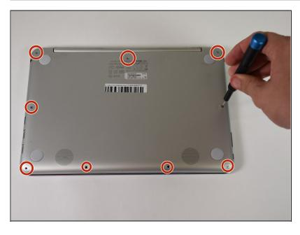
Use the T5 screwdriver to remove the nine 2.1 mm screws from the bottom of the device.
